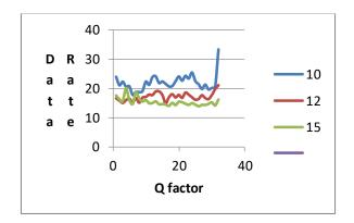
Figure: 15 Data rate versus Q factor for G656 SMF in the downstream
