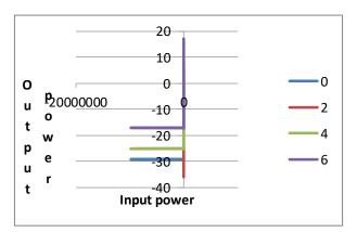
Figure: 21 Input power versus output power for photodetector PIN in downstream direction
