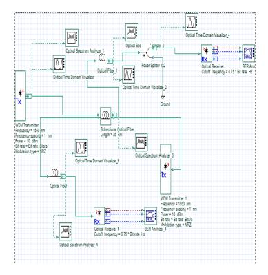
Figure 2: Simulation diagram for 1 user
