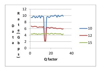
Figure:13 Data rate versus Q factor for G654B SMF in the upstream
