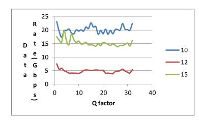
Figure:10 Data rate versus Q factor for G654A SMF in the downstream
