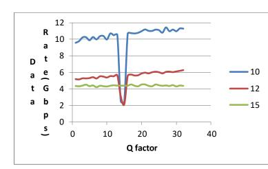
Figure: 16 Data rate versus Q factor for G656 SMF in the upstream
