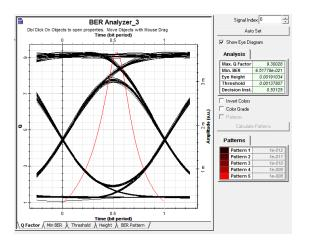
Figure 7: Eye diagram of G654 SMF operating at 10 Gbps with upstream direction and with a link distance of 10km for user 1
