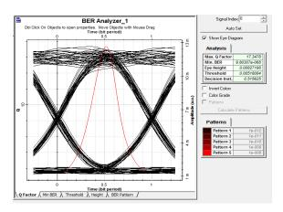
Figure 5: Eye diagram of G654 SMF operating at 12 Gbps with downstream direction and with a link distance of 10km for user 1
