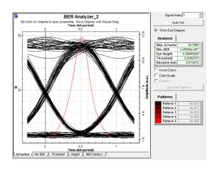
Figure 6: Eye diagram of G654 SMF operating at 15 Gbps with downstream direction and with a link distance of 10km for user
