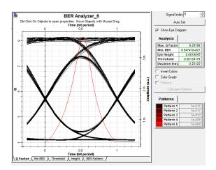
Figure 8: Eye diagram of G654 SMF operating at 12Gbps with upstream direction and with a link distance of 10km
