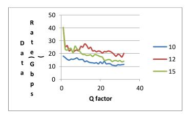
Figure: 17 Data rate versus Q factor for G657 SMF in the downstream
