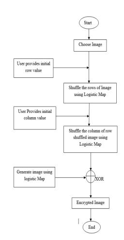
Here, user have choose image first and provide initial values for row and then shuffle the rows of Image using logistic map. And then user has to provide initial values for column shuffle. Shuffle the column of row shuffled image using logistic map and generate the image using Logistic map. Perform the XOR operation between Random Image and Shuffled Image then it gives output as Encrypted Image.
