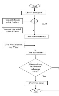
Here, first select the Encrypted image and generate Random image using Logistic map and perform XOR operation between random image and shuffled image. User has to provide initial column value for anti-column shuffle and also provide initial row value for anti-row shuffle. If the given initial value of row and column matches then we will get a Decrypted image s Original image. Else if initial values do not match then we cannot find an original image.
