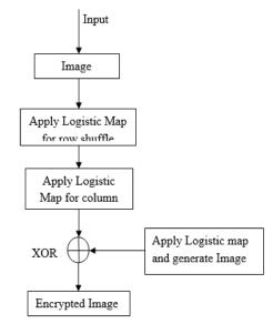
Taken input as secret image. First we are Reading an input image and it is going to generate some random values as M for rows and N for column. And we are applying Logistic Map for M generated random values for row shuffle. Similarly, applying logistic map for Column shuffle. Performing an XOR operation between the row and column shuffled image and generated random image for the Encrypted Image.
