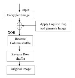
diagram shows the flow chart of Decryption Process. Here, it is exactly reverse order of Encryption process. Taking Encrypted Image as input, we are performing an XOR operation between the Random image and row and column shuffled image. Apply Logistic map for anticolumn shuffle and similarly apply logistic map for anti-row shuffle to get an original Image.
