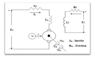
Fig.6.Equvivalent Circuit Of Separately Excited DC Motor
