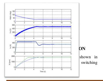
and low losses. Here SHP. 240V, 1750 rpm separately excited DC motor and additionally 300V DC supply are given to the field. To take the constant load of the circuit consider its kad 20Kg at constantly. In that simulation, there are four motor parameters are monitored by using displays, such as armature voltage, armature current, torque and speed of the DC Motor
