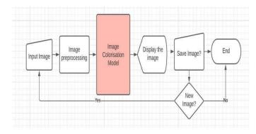
Fig -2: Software architecture
