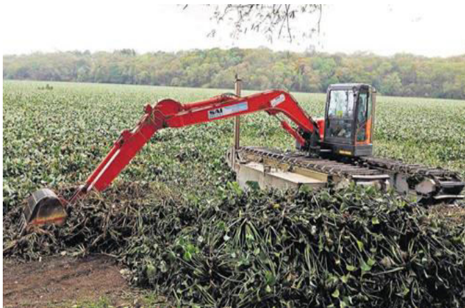
Fig. 4. Mechanical harvester for removal of water hyacinth
