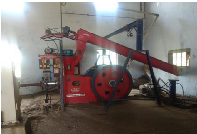
Fig. 6. Briquetting machine (Mainly designed to prepare briquettes from agricultural waste)
