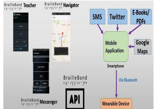
Fig 5: Braille band mobile application and integration of existing application
