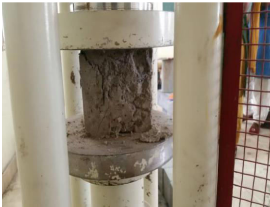
Fig.3 Geopolymer concrete cube after failure
