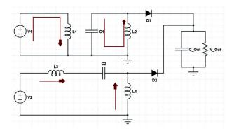
Fig -4: Equivalent circuit of DISEPIC in MODE 1
