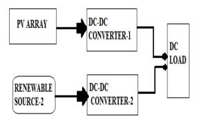
Fig -1: Block Diagram of Conventional System
