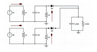
Fig -6: Equivalent circuit of DISEPIC in MODE 3
