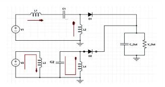
Fig -5: Equivalent circuit of DISEPIC in MODE 2
