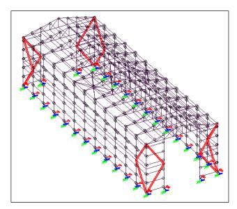
Fig 6: Single Diagonal bracing (Edge)
