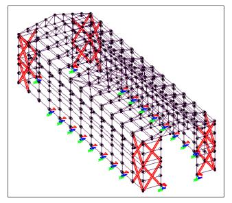
Fig 4: X bracing (Edge)
