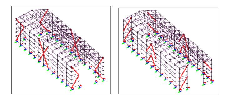
Fig 5: Single Diagonal bracing (center)
