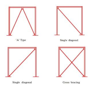
Fig. 2: Different Type of bracing Pattern
