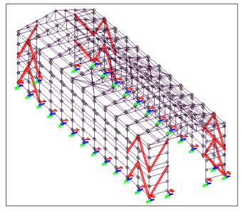
Fig 8: X bracing (Edge)
