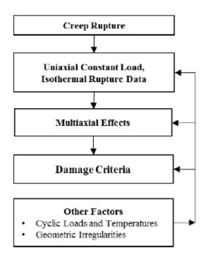
The time-dependent damage process that constitutes creep is mainly influenced by stress and temperature. Creep and stress-rupture tests are typically performed under isothermal uniaxial constant load conditions to determine the long-term damage effect on the material due to stress and temperature. However, similar conditions are rarely found in practical engineering problems where multiaxial stress states, cyclic or variable load and temperature conditions are often present.
