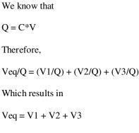
So, to improve the total output, we connected the piezo plate circuit connections in both series and parallel connection as combined. This improves the overall output and efficiency.
