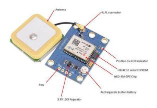
Fig-5: Neo 6M GPS Module
