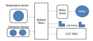
Figure 1: Block diagram for contactless temperature monitoring gate
