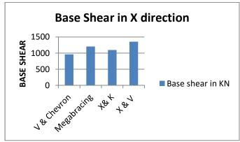
Fig -4: Base Shear in X direction
