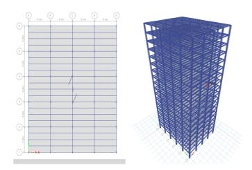
Fig -1: Plan and 3D view of steel bare frame
