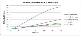
Fig -6: Roof displacement in X direction
