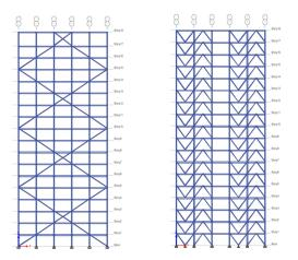
Fig -2: Elevation of Steel Frame with megabracing and Combination of Chevron and V bracing
