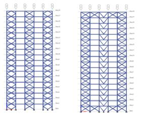
Fig -3: Combination of X and Knee Bracing & Combination of X and V bracing
