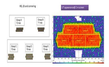
Figure 8.High Beam, Low Beam and Cornering LED
