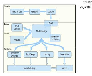
Fig 8 Commuter Aided Manufacturing Procedure
