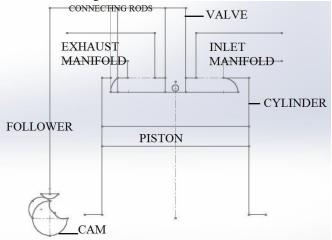
Fig: 4.1 Assembly of new engine
