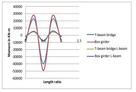
Graph 6.7: Moment for Wind load span 60 m bridge length.
