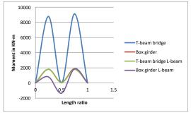
Graph 6.10: Moment for Live load span 80 m bridge length.
