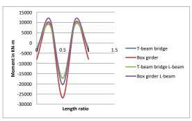
Graph 6.5: Moment for dead load span 60 m bridge length.
