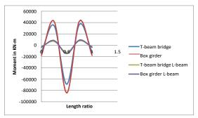
Graph 6.11: Moment for Wind load span 80 m bridge length.
