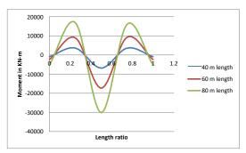
Graph 6.13: Moment comparison for different span of T beam bridge.
