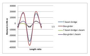
Graph 6.9: Moment for Dead load span 80 m bridge length.
