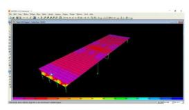
Fig 5.10: Dead load stress of Box Girder Bridge.
