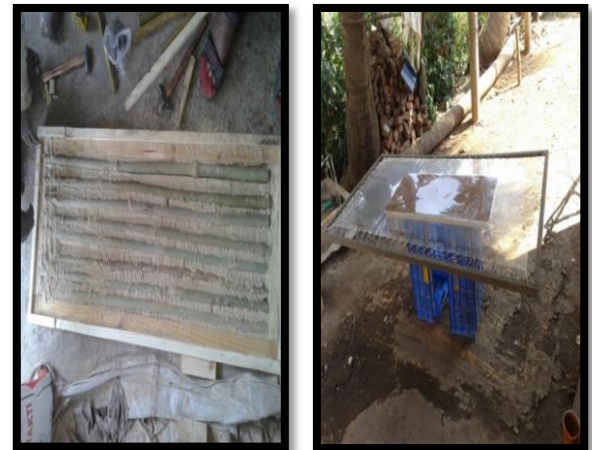
Fig -3 Making process of bamboo panel.
