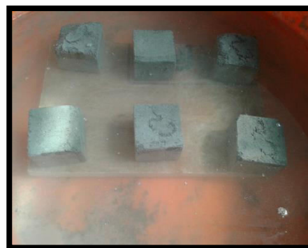
Fig No. 5 Water absorption for 24 Hrs
