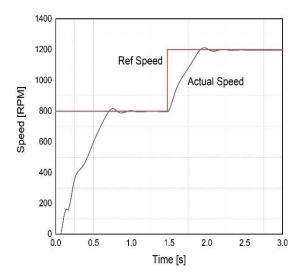
Figure 5.Step response from Standstill
