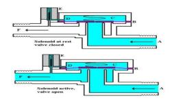
Fig.3. Solenoid valve operational principle.
