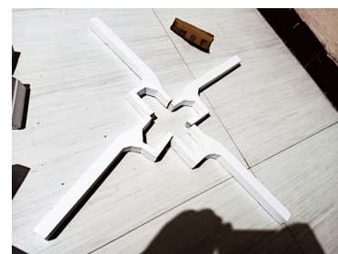
Fig. 18. Final 3D printed arms of hover bike chassis
