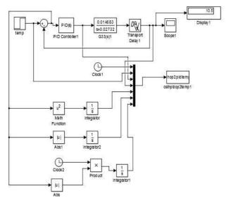
Fig 8 Simulink of PID for Temperature
