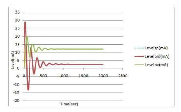
Fig. 7 Response of PID for level
