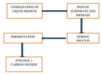
Fig 2 Block diagram of CSTR
