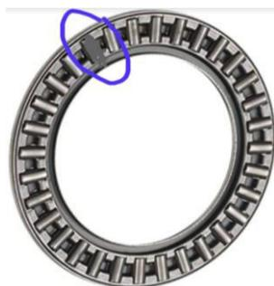
Figure3: Rejected bearing
