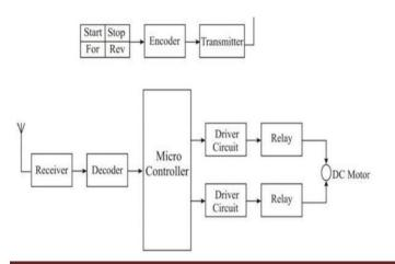
It is used in order to start or stop the entire operation of the object lifting jack generally remote switch is used to operate motor in reverse and forward direction. The remote switch is a class of electrical switches that are electronically actuated. This is designed to provide the simultaneous actuation of multiple sets of electrical contacts, or the control of direction of electric current.
