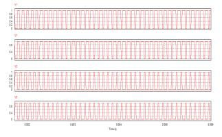
Fig.6 (i) switching pulse waveform during short circuit condition
