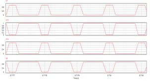
Fig.6.2 (e) pulse waveform for S1, S2, S3, S4
