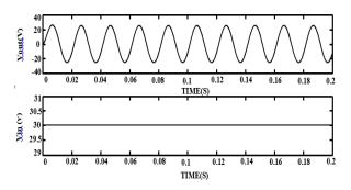
Fig.6.1(a) Input and Output voltage of single phase spwm inverter in open loop system
