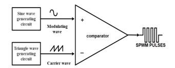
Fig.1 (a) Sinusoidal Pulse Waveform Generation
