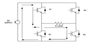
Fig.3 (a) current flow path in Mode 1
