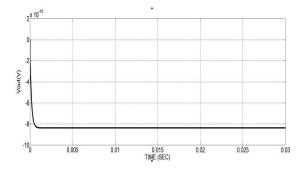
Fig.6.4 (a) output voltage waveform of single phase SPWM inverter with shoot through fault protection
