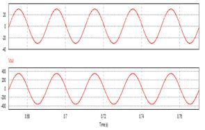
Fig.6.2 (f) output voltage and current waveform of single phase SPWM inverter with filter
