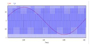
Fig.6.2(c) Sine and Triangular Wave Comparison
