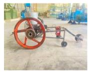
metering device ,seed tube ,disc type bed former, runner wheel, handle and power transmission system. Seed hopper contains the seed and the seed metering device. The amount of seed contained depends upon the size of the seed hopper. The seed rate and seed spacing are
