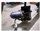
Figure 2.5 Wiper Motor
