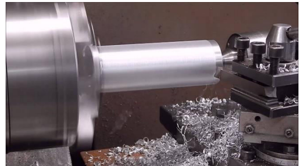
Lathe turning of shaft
