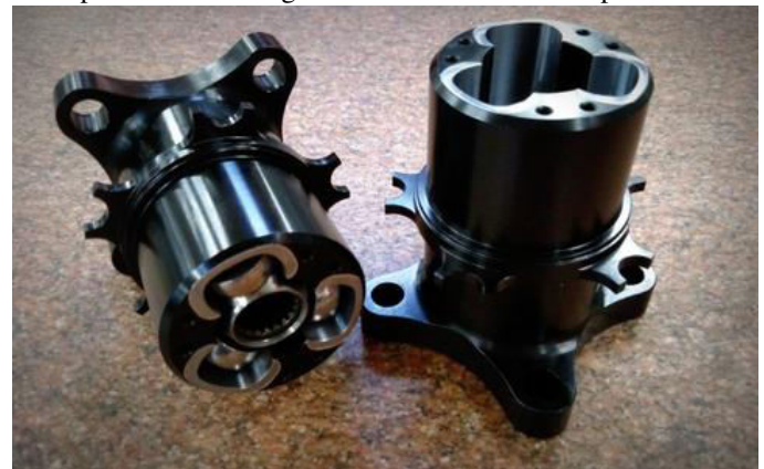
Hubs fabricated with CNC
