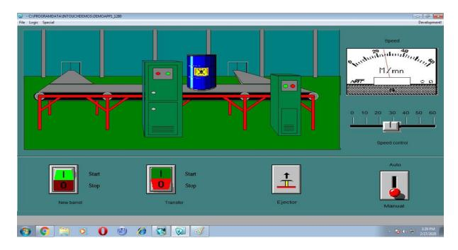
•When the Labelling process is completed then the Ejector pushes the barrel using the Ejector switch and if the ejector doesn't operates then the barrel gets damaged and a message is displayed on the Screen .
