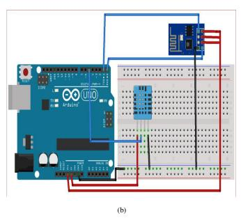
Fig -4 Arduino Interface with (a)Soil Moisture Sensor and (b) DHT11 Sensor
