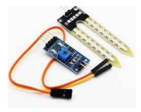
Fig -2 Soil Moisture Sensor
