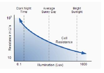
Fig -6 Experimental Result of LDR
