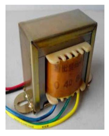
Landscape lighting, however, is typically supplied in lower voltage (12 Volts) spread out through several different lights. A **transformer** can convert the 120v electrical currently supplied from your house down to the **12v** needed for each low voltage landscape lighting fixtures in your lawn!
