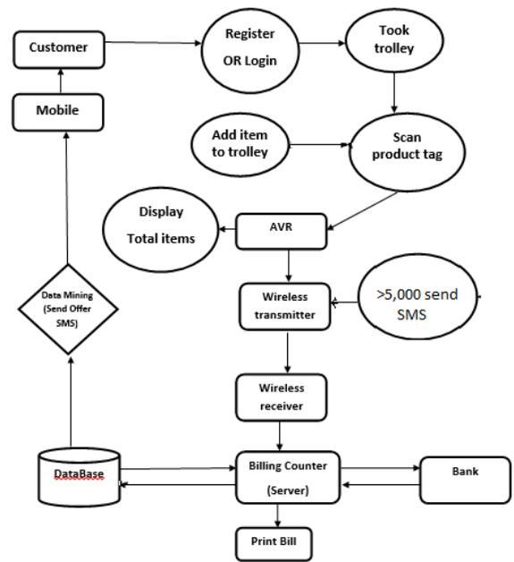
Fig.2 Architecture of automatic billing trolley
