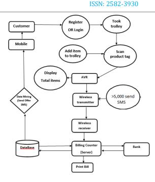
Fig.2 Architecture of automatic billing trolley
