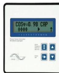
APFC relay is connected to a 3 phase + neutral 440 volt system. The motor And capacitor are also connected to the same system . Relay is given the current of one phase(L1) through CT and given system voltage (L1-N)..so above relay is used to turn on 6 capacitor
