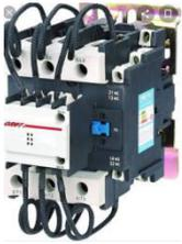
Operation principle of a contactor. The current passing through the contactor excites the electromagnetic. The excited electromagnet produce a magnetic field, causing the contactor core to move the armature. A normally closed (NC) contact completes the circuit between the fixed contacts and the moving contacts.
