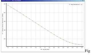
12: Shear stress variation with coil diameter
