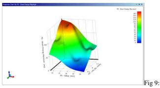
Response Surface for strain energy using E glass
