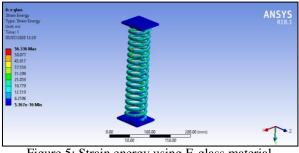
Figure 5: Strain energy using E-glass material
