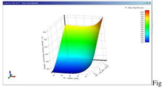
8: Response Surface for shear stress using E glass
