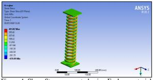
Figure 4: Shear Stress generated using E-glass material
