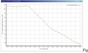
14: Strain energy variation with respect to coil diameter
