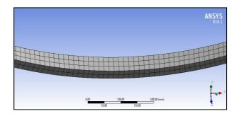
Figure 3: Meshed model of leaf spring
