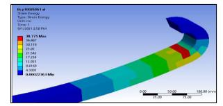
Figure 8: Strain energy plot of mono leaf spring using aluminium composite material
