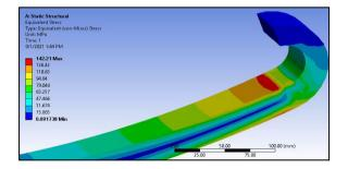
Figure 5: Equivalent stress plot for steel
