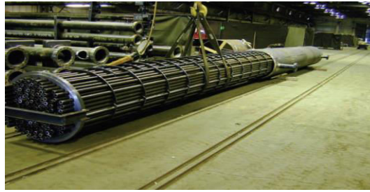
Fig 3- Tube bundle and insertion
