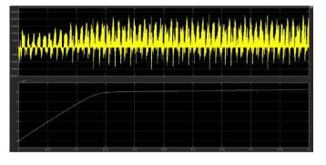
Figure-4. Output voltage and current of boost converter
