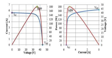
Figure-2. MPPT Curve of a PV Cell
