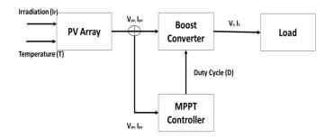
Figure- 1. Block Diagram of Solar Modules
