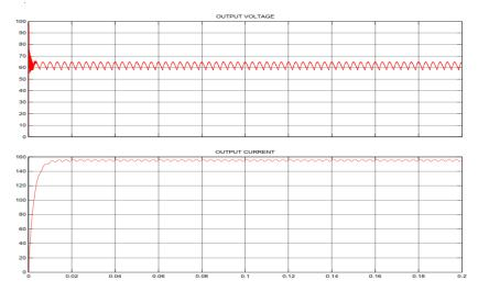
Figure.3.2 output waveform of load voltage and load current of welding machine
