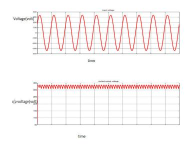
Figure.3.1 waveforms of ouput voltage for 3-phase rectified voltage
