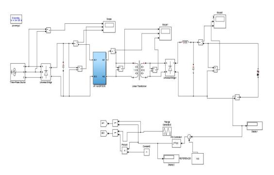
Figure.3 simulationwelding circuit in constant current mode of 3-phase, 60volt, 100 ampere
