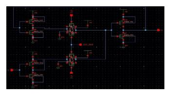
Figure 3 A positive MUX-based D-latch using transmission gates
