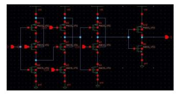
Figure 4 a real Single Phase Clocked Latch
