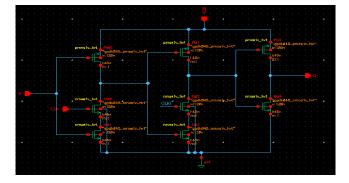
Figure 5 a real Single Phase Clocked Latch with split output
