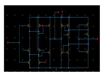
Figure 7 Test bench for the 1:2 Deserializer circuit
