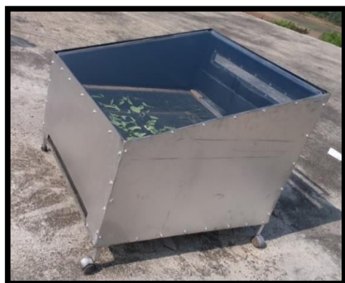
Fig. 2 Pictorial view of solar cabinet dryer Fig. 3 Thermophilic view of solar cabinet dryer
