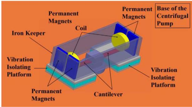
**Fig-6:** Proposed design of the VEH (a) Top view (b) 3D View of the VEH [3].
