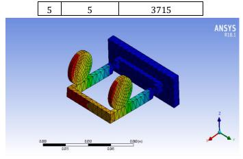
Fig- 8: Analysis result at 552 Hz frequency (mode 1)
