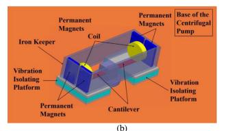
**Fig-6:** Proposed design of the VEH (a) Top view (b) 3D View of the VEH [3].
