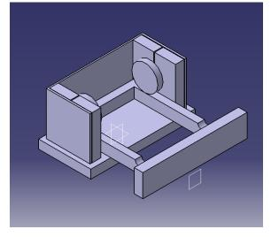
Fig-7: Final model of system with compliant mechanism in Catia.
