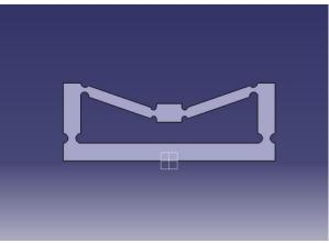
Fig-1: Symmetric Five bar Mechanism
