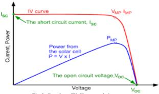
Fig.3: Graph on IV-Characteristics
