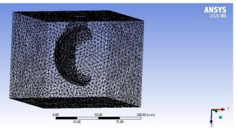
Fig -3: Turgo Turbine blade Meshing
