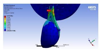
**Fig -5**: Meshing and Structural analysis of blade
