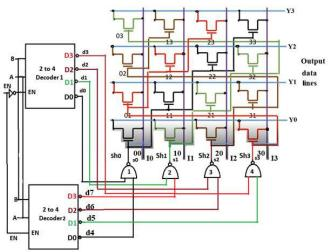
Fig.2. Decoder & NMOS Based Bidirectional Barrel Shifter
