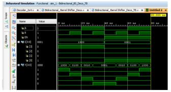
Fig.3(a). Simulation Output Waveforms for proposed Bidirectional barrel shifter
