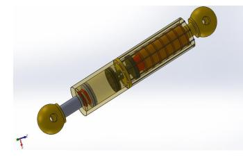
Fig-11: Regenerative shock absorber assembly with generating module
