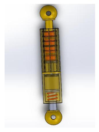
Fig-12: Regenerative Shock Absorber assembly front view
