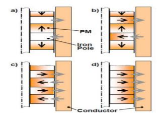
Fig-5: Different configurations of magnetic array
