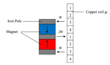
Fig -7: 3 phase power generation concept
