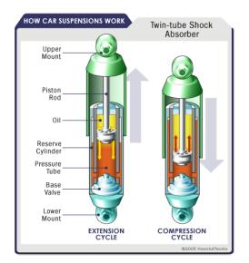
Fig -1: Working of Shock Absorber (Image courtesy: howstuffworks.com)
