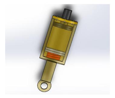
Fig-10: Cad model of Monotube shock absorber without generating module
