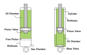
Fig-2: Monotube and Twin tube shock absorber (Image courtesy: <u>www.tein.co.jp</u>)
