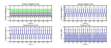
**Fig -9:** Combination of graph for oscillation frequency = 20 Hz and initial velocity = 3 m/s
