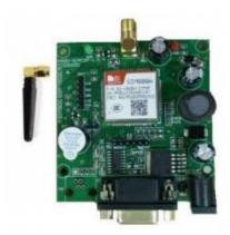
GSM means Global system module is used for communication. A sim card has to be inserted for communication. Messages can be received for defined number using sim card. Time Division Multiple Access method is used for this process. It can communicate mobile, Computer over a network. It can also be connected to the computer through Bluetooth or serial ports. It has the abilities to make a call or send a message and it can delete messages also in the SIM card that are received or send by the GSM.
