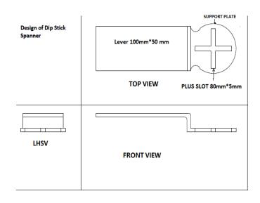
Fig 3: 2d Design of Dip Stick Spanner.
