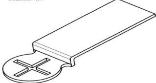
Fig 2: 3d Design of Dip Stick Spanner.
