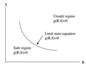
Fig:- Limit state showing failure surface, safe and unsafe regions
