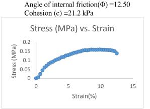
Fig:- unconfined compressive strength test results in form of stress vs strain
