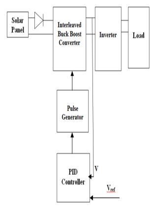
Fig. 1. Proportional Integral Derivative Controller in Photovoltaic interleaved buck boost converter for solar system
