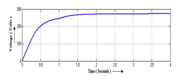
Fig. 5. DC link voltage waveform of Converter Output
