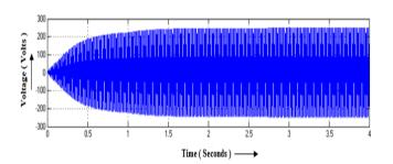
Fig. 6. Output voltage of inverter with PID controller
